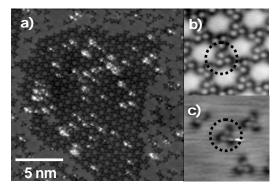
Fig. 1 STM image of self-assembled glycine molecules on a Cu(111) ( $V_s = -0.5VI = 1.0 \text{ nA}$ )
