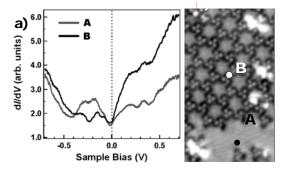
Fig. 2 (a) d*I*/d*V* spectra of a Cu(111) substrate (A) and a hexagonal area surrounded by glycine trimers (B) measured at the points indicated by A and B in (b), respectively.
